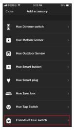
Step 3: Tap a brand to select it, any brand will work. Then operate the switch as instructe to enable it to be added to the Hue Bridge.
