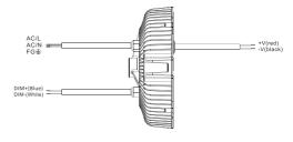
Contact DIM+and DIM- with 1-10V dimmer
