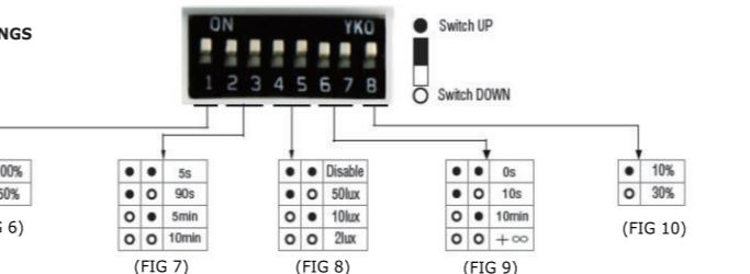
**Detection Area** - It can be adjusted by combining DIP switches for specific application [FIG 6].
